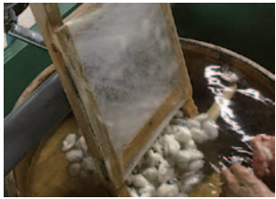
繭を広げる繭むきは、熟練の職人でも1日に500gが限度の根気の要る作業。 Spreading wet cocoons. Maximum volume by a skilled artisan will be 500g a day. Extremely hard work.
